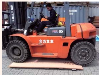
Simulated loading test by 8 tons forklift by our Storekeeper in IQC program
