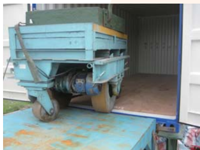
7,260kg loading test for Brigantine container floorboards
