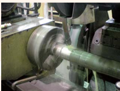
Cooling Pipe being ground
