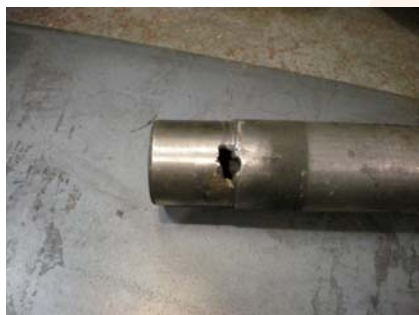
Damaged Cooling Pipe
