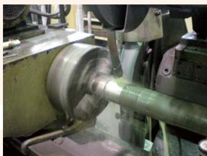
Cooling Pipe being ground
