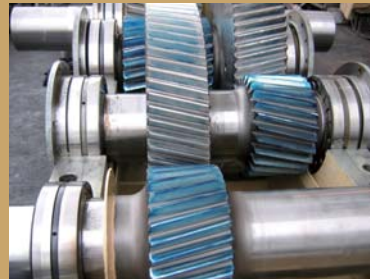
Fig 3. Check for gear contact pattern
