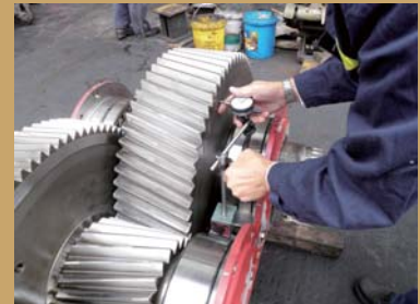
Fig 4. Measurement of perpendicularity of gear
