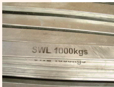
Safety Working Load is marked on each beam
