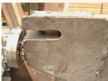
Hangerbeam after test—left & right—no deflection, no sign of damage/crack on notch and weld bead
