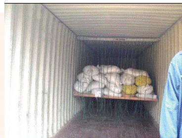
Hang the sand bags onto the beam
