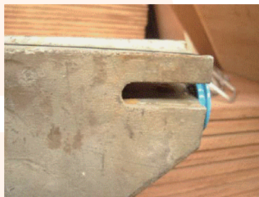
Hangerbeam after test—left & right—no deflection, no sign of damage/crack on notch and weld bead
