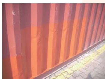
Straightening of side panel
